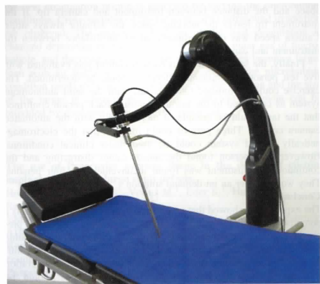
Fig. 1 SOLOASSIST is a mechatronic system that aid camera guidance during a minimally invasive surgical intervention. This system allows a 360° circle range in conjunction with an 80° inclination of the endoscope.
