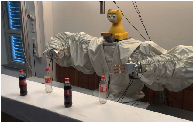
Figure 5: In the BIMANUAL scenario, a camera is used to recognise empty bottles which a bimanual robot should remove from the table to a “dishwasher” location on the left side, behind the table (Gaschler et al. 2013a; Giuliani et al. 2013). A video of the robot operating in this scenario is available at http://youtu.be/yMmZkhHr8ss .
