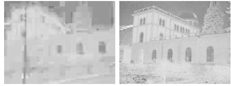
Fig. 2. The color information (hue) in low quality JPEGs is unreliable (left), compared to this information in a high quality image of the same object (right).
