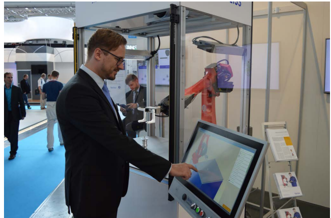
Fig. 1: The redesigned user interface running on an industrial touchscreen next to the robot workcell. The main focus is on ease-of-use for workers in small and medium-sized enterprises with small lot sizes.
