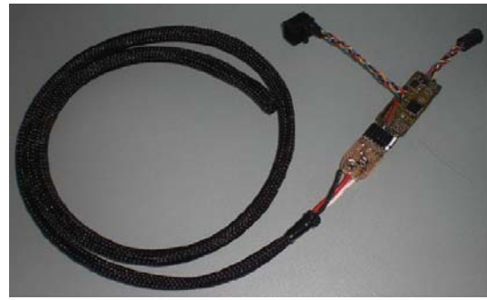
Fig. 9. Hand-Crafted Prototype of Cable in a Flexible Hose with MCU
