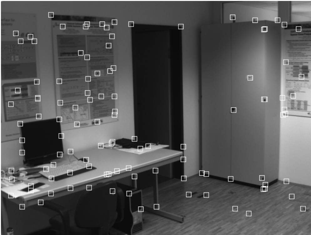
Figure 4.1: An example of the results of the Shi and Tomasi corner detection algorithm. The rectangles refer to points that the algorithm identified as corners. Before the corner detection was run, the image was divided into a grid with cells of the size 30x40 pixels. Only the maxima within those cells is plotted.
