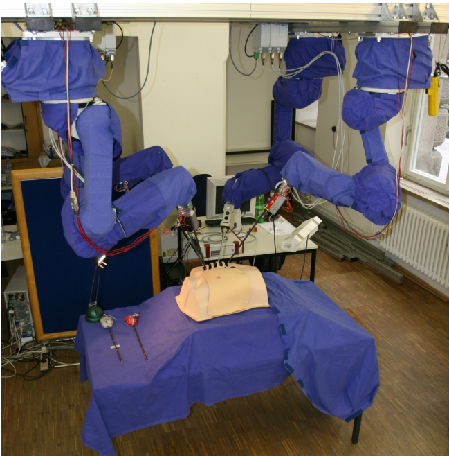
Fig. 1. Hardware Setup. Ceiling mounted robots with surgical instruments
